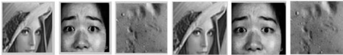
Figure 8. Grey level of original image and watermarked image under cropping attacks and the corresponding qualities: (a) Lena (38.7569 db), (279.3277 db), (b) Facial (35.2695 db), (283.9997 db), (c) Moon (36.3759 db), (271.2718 db).
