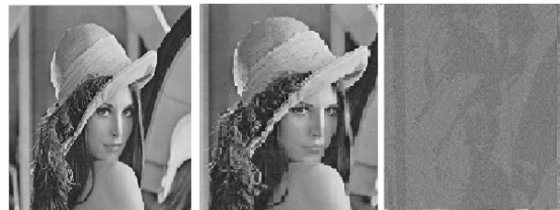
Figure 1. Reconstructed image, compression image and quantization image by using DCT.
